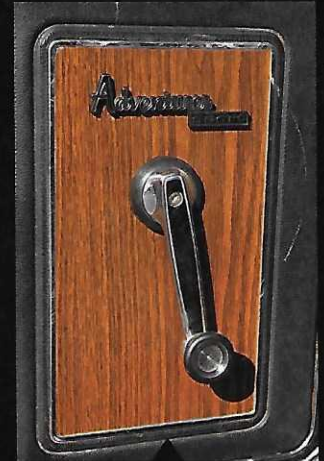
In later years, Dodge moved its window cranks out from the door panels so as to avoid the small scar seen here on the driver's door panel.
