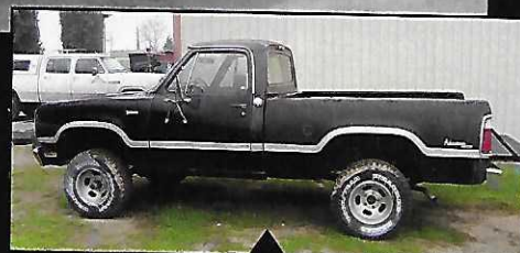
The Bledsoes’ 1974 W-100 Power Wagon was not so shiny when Sam Bledsoe brought it home in 2008. The plug in the gas filler hole is a factory item. On two-wheel-drive models, the gas tank was in the frame with the gas cap on the box side.
