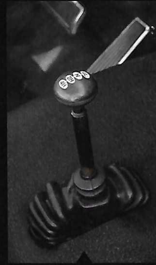
The NP 205 transfer case is conveniently controlled by a single lever.
