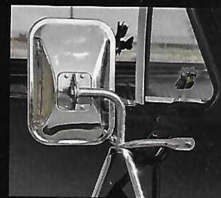
The original stainless steel, 6x10-inch, low-mount mirrors were polished at the time the truck was refurbished.
